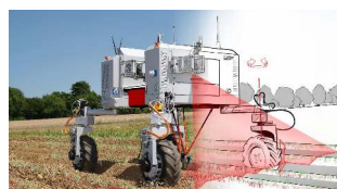
BoniRob ® equipped with delta robot for mechanical weed control
