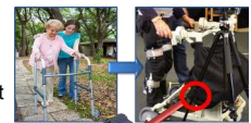
A robotic prototype equipped with a Hokuyo Laser Sensor aiming to record the gait cycle data of the user (below knee level).
